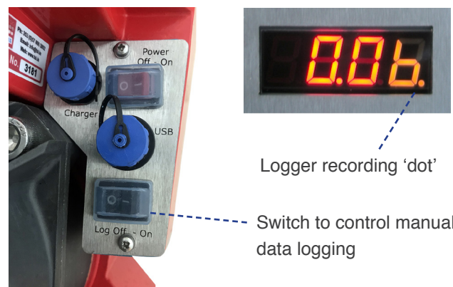
Fig. 3.6 Activating data log. The picture on right hand side shows that the logger is recording. This is indicated by the orange 'dot' on the bottom right
