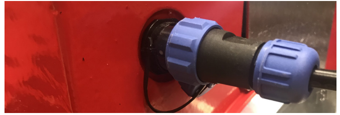
Fig. 5.1(b) Flowmaster battery charger socket (casting) NB. This charging socket may not be on your model
