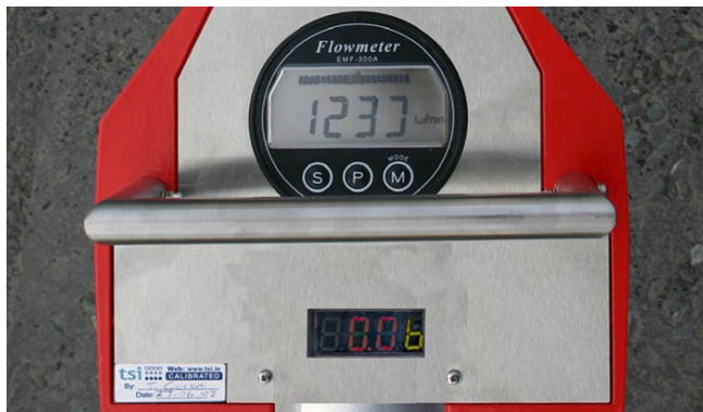
Fig. 4.2 An example of a flow readout and a residual pressure reading. Photograph courtesy of Laois Fire Service.
