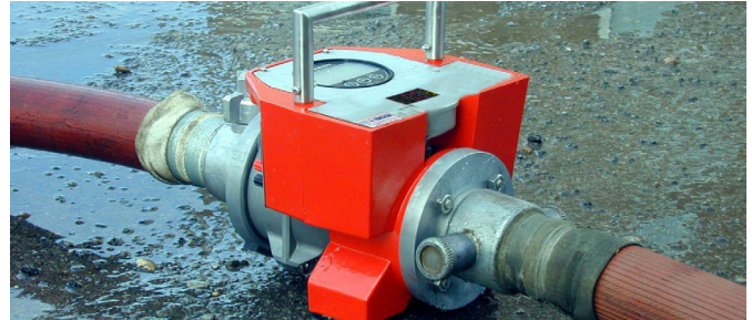
Fig. 4.4 Inline use of Flowmaster. Photograph courtesy of Essex County Fire and Rescue Service
