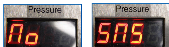
Fig. 5.3 This is how No SNS (flow sensor not connected) is displayed on the LED readout
