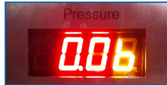
Fig. 3.5 After 3 seconds, LED readout displays pressure in bar. The letter 'b' in image indicates the units are 'bar'
