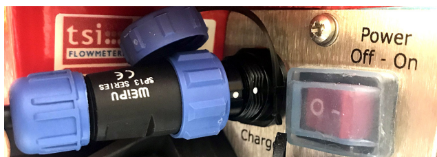
Fig. 5.1(a) Flowmaster battery charger socket (power panel)
