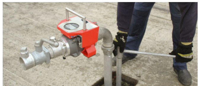
Fig. 4.6 Caution! Never allow the Flowmaster to be used in an open-ended position. It is essential to secure the Flowmaster so that it cannot move about freely
