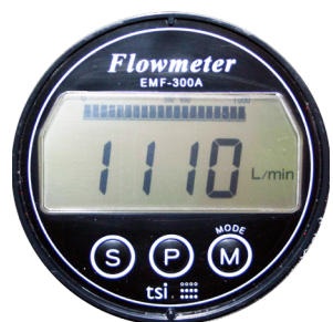
Fig. 3.2 Flow meter display when ready for flow measurement, water is filling the pipe and is flowing
