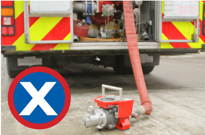
Fig. 4.6 Caution! Never allow the Flowmaster to be used in an open-ended position. It is essential to secure the Flowmaster so that it cannot move about freely
